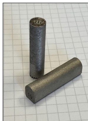
Fig. 2. Vertical and horizontal tensile blanks.
